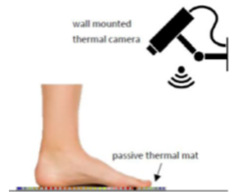
Figure 2: Schematic of the Bath Mat device
